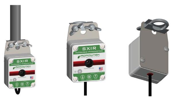
Mount the bracket to the back of the sensor using the included screws. The u-bolt clamp can be secured to 1/2" EMT or PVC conduit, shelving poles, etc., or use the bracket holes to mount to a tripod, etc.
