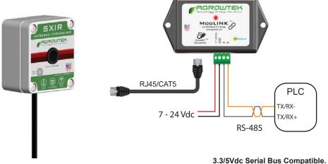
Include required bus terminating resistors per EIA standard.
