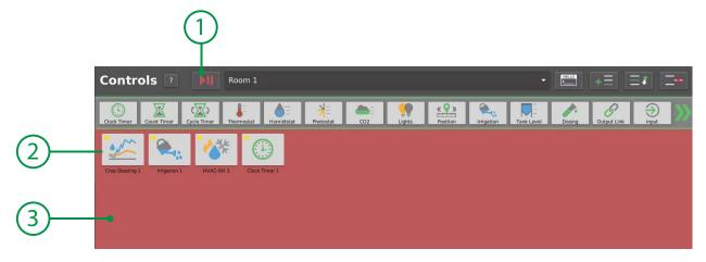
When the control group is in Maintenance mode, the run/pause button (1) remains green. The function icons status dot (2) will turn Red if no maintenance rules exist in the function. The background will turn yellow to indicate the workspace is in maintenance mode.
