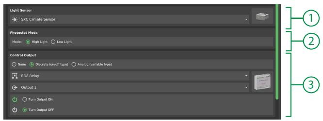
1. Sensor Device Select a sensor device (or average) for the light function to read.
