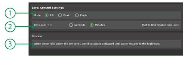
1. Mode FILL: Fill valve opens when low level is dry until high level is wet.
