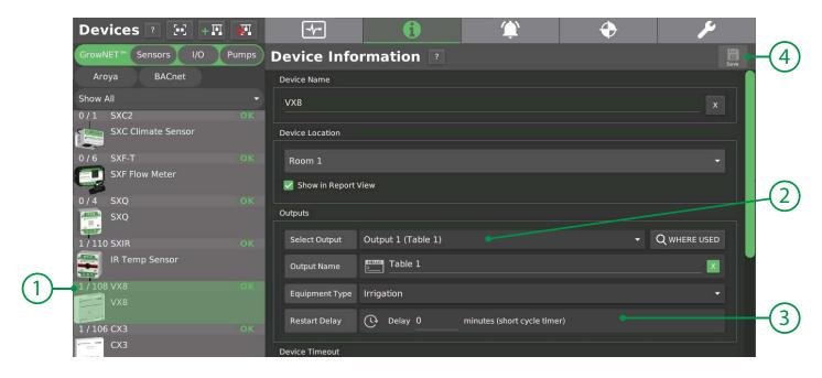
When the output turns off and the restart delay timer is active, the output status will be shown in RED.
