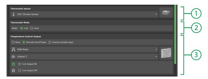
1. Sensor Device Select a sensor device (or average) for the thermostat function to read.
