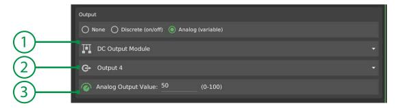
1. Device Select the GrowNET™ device that the output is located on.
