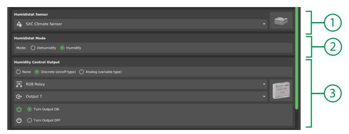
1. Sensor Device Select a sensor device (or average) for the humidistat function to read.
