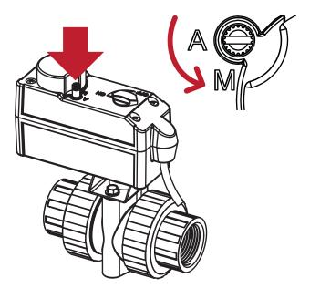
1. Press the operation selector down then rotate until the slot in the knob is aligned to the M position.
