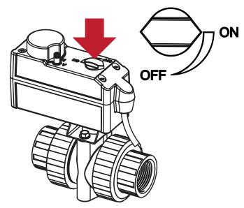
2. Rotate the position knob with a 10mm open end wrench.
